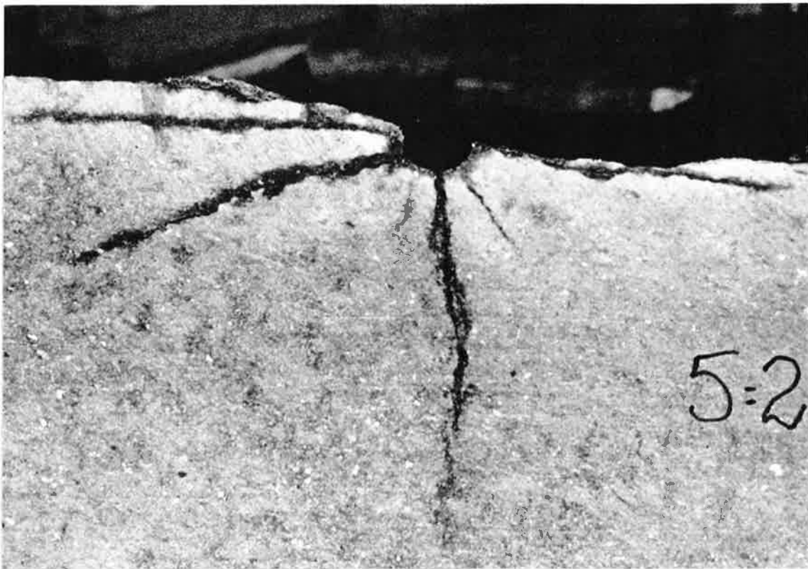
Figure 1: Radial cracks behind 51 mm blast-hole, Olsson and Bergqvist (1993a).
