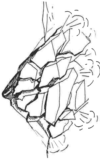
Figure 2. Hole in wall stope with a powerful charge.
