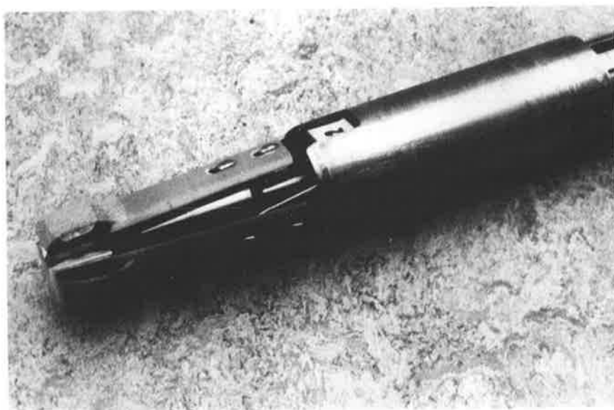
Figure 2. The strain gauge tongues mounted to the equipment.
