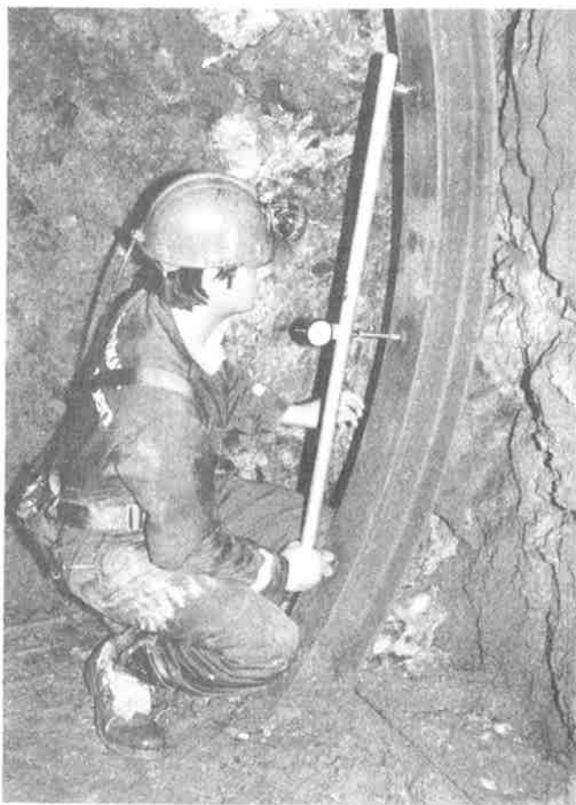
Figur 5 Stålbågarnas radiella deformation kunde mätas med en Curvometer. The change in curvature of the steel ribs was measured with a Curvometer.
