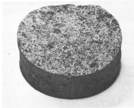
Fig. 3 Brott i kontaktytan. Failure in the contact surface.
